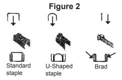
Load the staples or brad nails into the Staple Channel. Each of the fasteners is to be loaded into the Staple Channel with its sharp end facing the base of the Staple Channel-see Figure 2.
